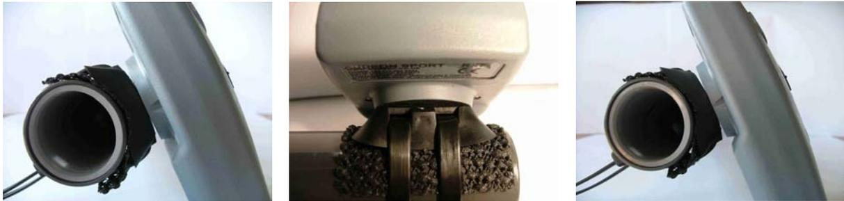
in use due to the stress placed on the central mounting screw hole. This occurs when users try to move the receiver whilst exercising.
