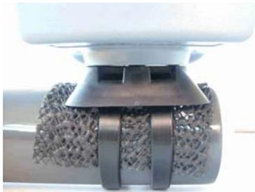
**Correctly** fastened to a round bar using 7.6mm cable ties, a non slip mat and the inner mounting holes - no distortion of the bracket. The bracket must be securely fastened on to the exercise equipment to prevent the users "playing with it" and the wires coming loose and fracturing.
